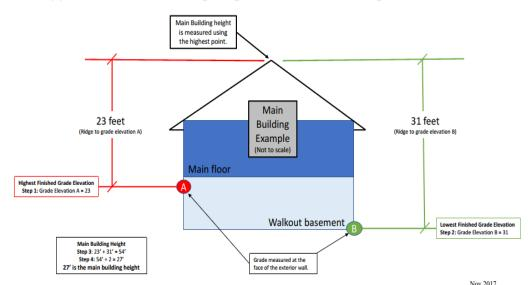
Appendix A: Main Building Height Measurement using Grade Elevation
